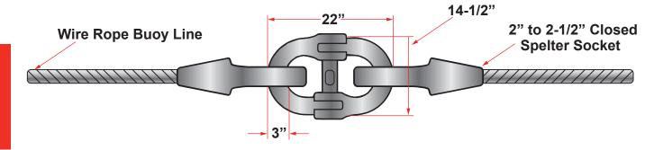
The 110-ton S.W.L. Hinge Link is specifically designed to provide a single, fast, easy connection to spelter sockets or thimbles that will hinge when passing over a wire rope drum. Hinge Link can be used to connect up to 3'' wire rope closed spelter sockets and thimbles on anchor pendant lines.
